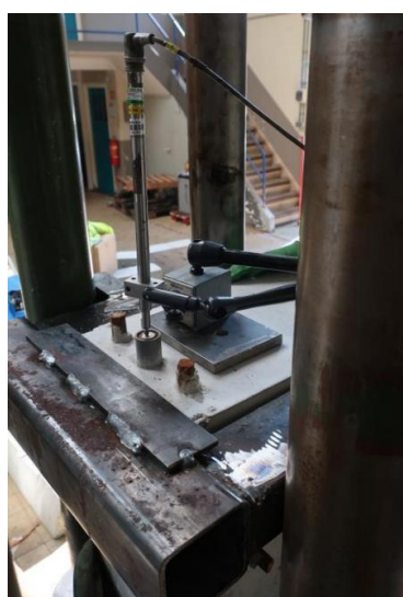
Attachment LVDT topside
