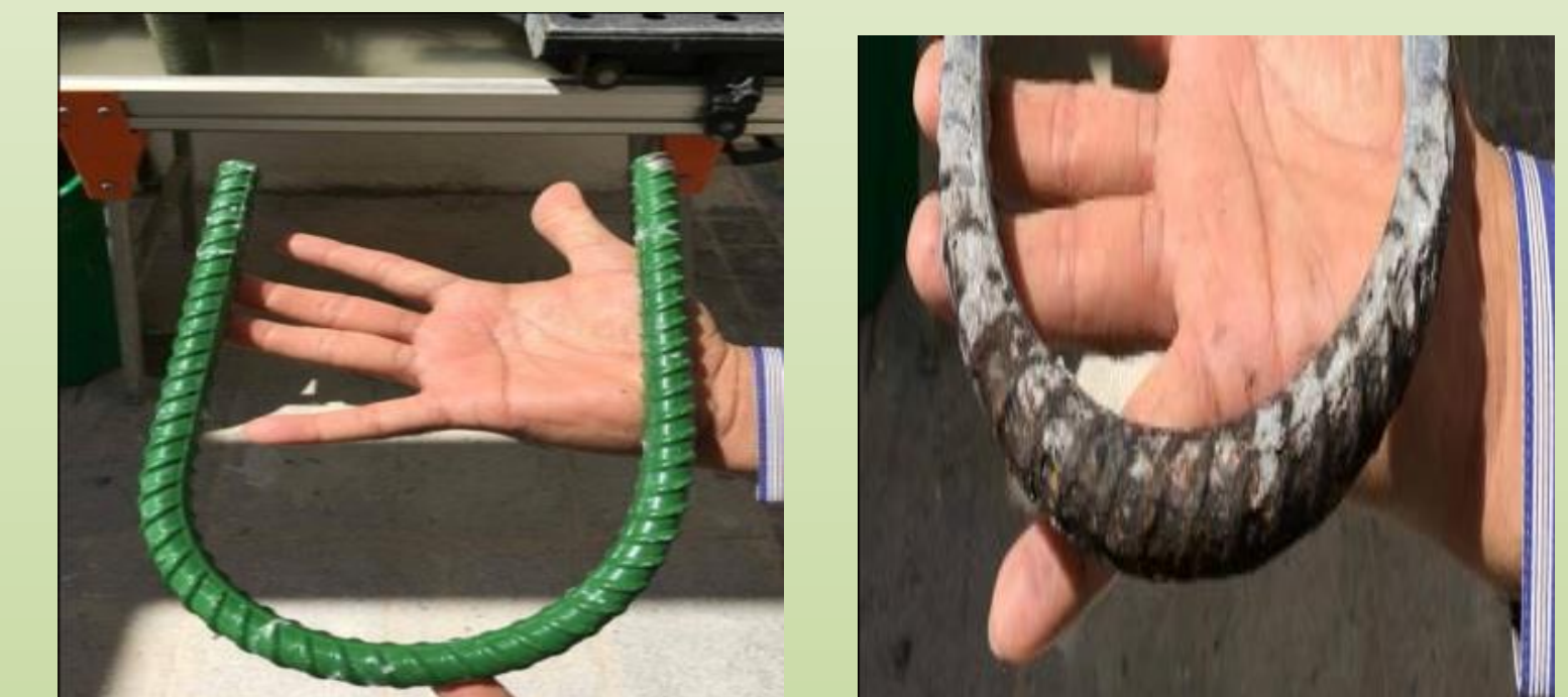
Figure- 8 The extracted steel bars from samples after 2 years of submergence in sea water. Severe corrosion was present at mild steel while no corrosion was found at epoxy coated rebars.
